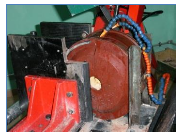
Cutting mine in half on bandsaw
