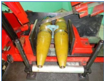
Large calibre being cut in half
