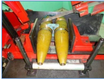
Large calibre being cut in half
